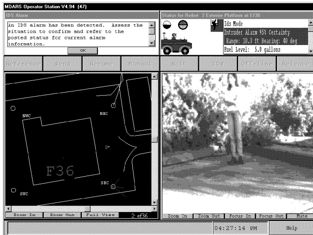
Figure 5. MRHA Operator Station Display depicting an IDS Alarm for exterior robot #2.
